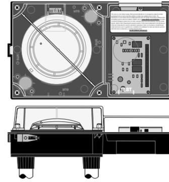
Duct Detector Housing, Front and Bottom View
