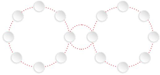
ES Net eases design and installation by supporting ring, star, bus and bridged ring network topologies. Because you can combine multiple topologies, you can create fault-tolerant, highly survivable networks while mixing and matching media between nodes to optimize cost, distances and performance.
