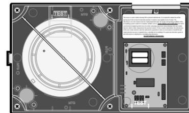
In-Duct Housing with 4098-9714 Sensor
