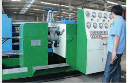
Valve Pressure Testing Machine (Horizontal)
