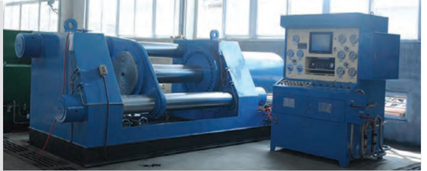
Valve Pressure Testing Machine (Horizontal)
