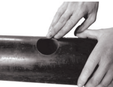
1. Pipe preparation Clean the gasket sealing surface within 16mm of the hole and visually inspect the sealing surface for defects that may prevent proper sealing of the gasket. Don't drill the hole on weld line.
