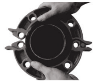
4. Housing installation Remove bolts and nuts, place two housings over the gasket, making sure the housing keys fit into the pipe grooves. Re-insert the bolts and hand tighten the nuts.
